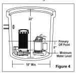
The on level of the Electrical Primary Pump must turn on before the 11 inch on point of the AC/ DC Sump Pump. Do not raise the AC/ DC Sump Pump above the level of the Electrical Primary Pump.
